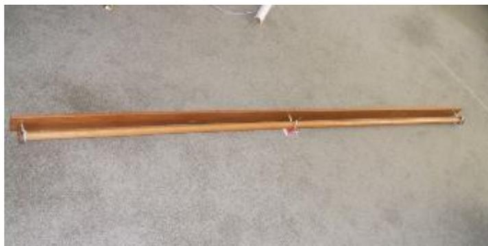
5. Pre drill the back board with a fairly large drill (you do not want to split the board) and screw the hooks into position. The ones I use I screwed up to the end of the thread. Then, using a hack saw, cut off the thread that is protruding through the back.
