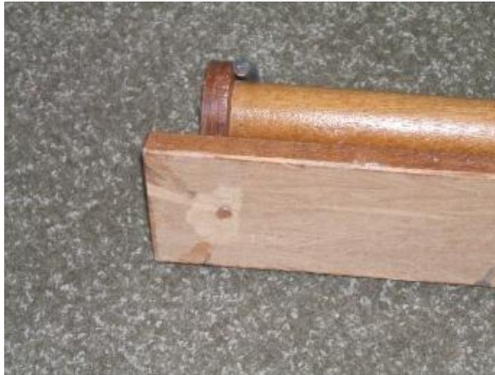
6. If you are using wooden discs cut these and screw to each end of the dowel.
