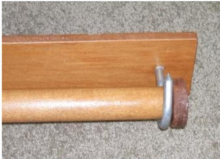
3. The timber back board I used was 65mm/2½in x 20mm/¾in.
